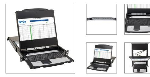
DisplayPort KVM switch allows complete access and control of 8 DisplayPort computers or servers using one monitor, keyboard and mouse.
